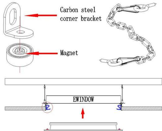
Eighth: Lockup the steel chain by the retaining rings on front frame and holding frame, then fix front frame by magnet and carbon steel corner brackets.
