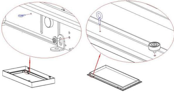
Seventh: Fix 2 retaining rings on opposite angles of holding frame and 2 on front frame in corresponding side.
