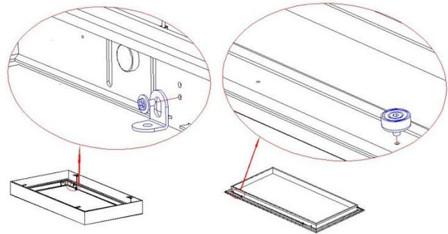
Sixth: Fix 4 Carbon steel corner brackets on holding frame and 4 magnets on front frame.
