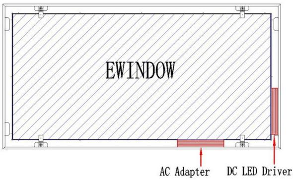
Fifth: Put AC Adapter and DC LED Driver inside the holding frame.
