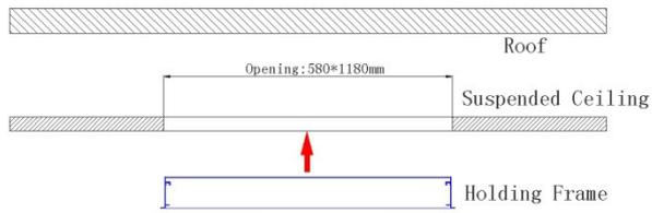
First: Open a 580\*1180mm hole on suspended ceiling, and drill four  $\Phi 10$ mm holes on roof.
