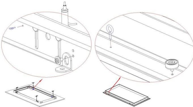
Seventh: Fix 2 retaining rings on opposite angles of holding frame and 2 on front frame in corresponding side.
