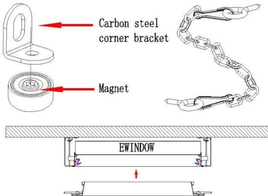
Ninth: Lockup the steel chain by the retaining rings on front frame and holding frame, then fix front frame by magnet and carbon steel corner brackets.
