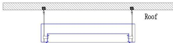
Second: Fix holding frame on steel strings.
