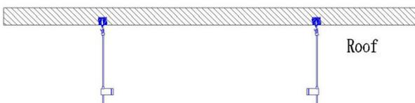
First: Drill four  $\Phi 10$ mm holes on roof (4 points of rectangle 624\*916mm). And fix 4 steel strings.
