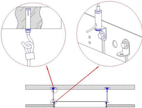
Third: Hang up the holding frame to the roof by 4 sets of steel string components
