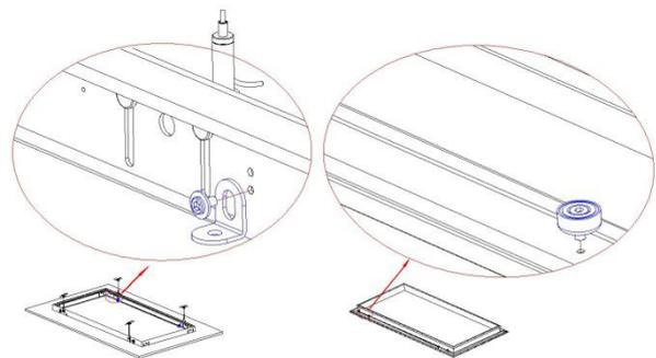
Sixth: Fix 4 Carbon steel corner brackets on holding frame and 4 magnet on front frame.
